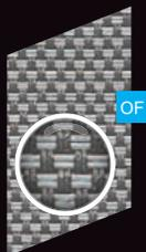
**OF** OPENNESS FACTOR (T<sub>vnn</sub>): relative area of the openings in the fabric (hole). It is considered as independent of the colour. For fabrics with the same weave, it should be measured using the darkest colour in the range.
