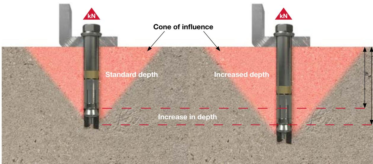
The above diagram shows how increasing the effective embedment depth of the anchor achieves a greater cone of influence and a greater resistance from the concrete which results in a greater tensile resistance from the anchorage.
