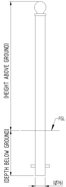
Functional yet striking, the GFC2000 bollard is manufactured from mild steel and galvanised for longevity. A spherical cap is welded on to the bollard to complete the design. This bollard is ideal for providing an aesthetic solution to unauthorised parking and access.
