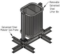
The AUTOPA 'HVM LITTER BIN' has been designed to be installed where pedestrians and vehicles could share the same area and has the ability to be removed if necessary to allow access.
