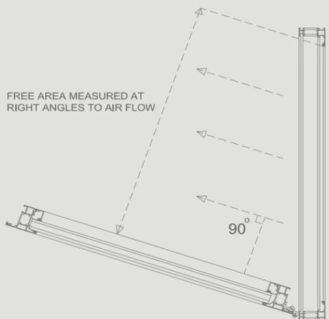
FREE AREA MEASURED AT RIGHT ANGLES TO AIR FLOW
